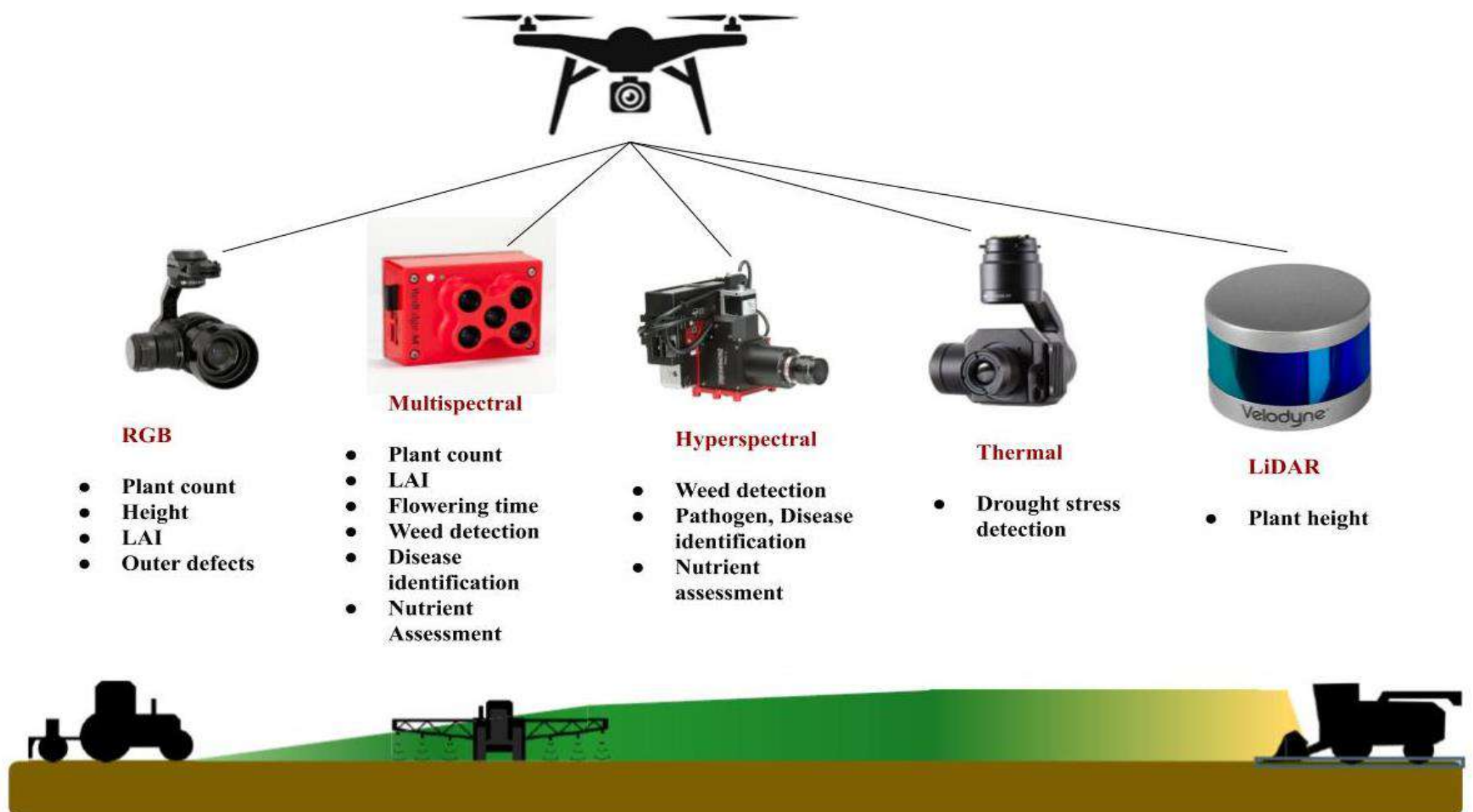
Figure 1: Sensors integrated with UAV and their application in Agriculture
